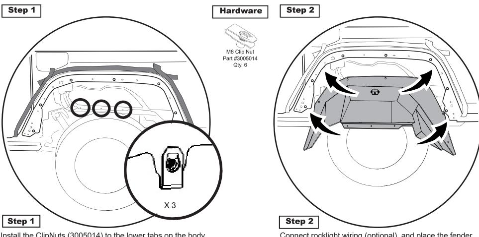
Install the ClipNuts (3005014) to the lower tabs on the body sheetmetal of the JT Wheelwell. Three (3) clips per side will lineup with the holes in the wheel well liners. Simply Press on the clips as shown in the detail to the right.
