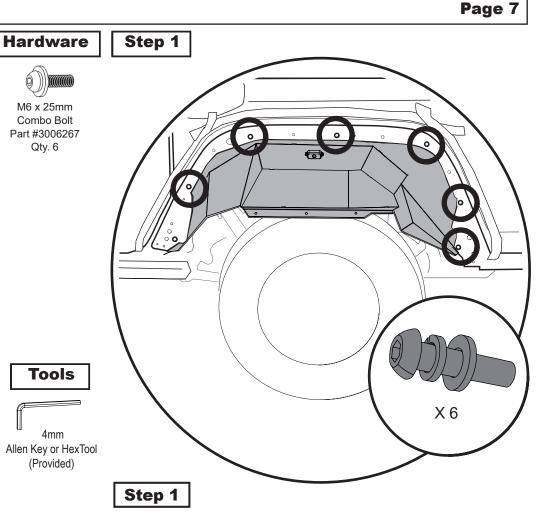
If you are NOT installing Bestop flares, or you have another solution, go ahead and hand install the Combo bolt (3006561) into the remaining holes of the JT Wheel well. Six (6) bolts per side. Make sure to check and lineup body holes with the threaded insert holes in fender liners.
